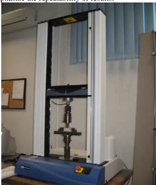
Fig 5.3 Test bench used in the three-point bending tests.
