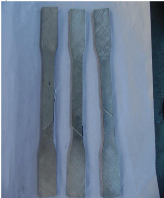
Fig 3.6 Specimens after Tensile Testing
