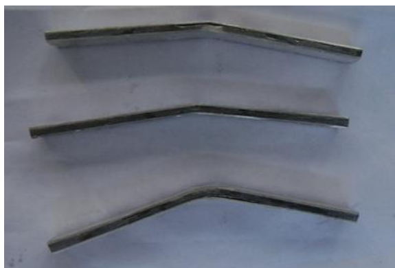
Fig5.5 Specimens after Flexure Test
